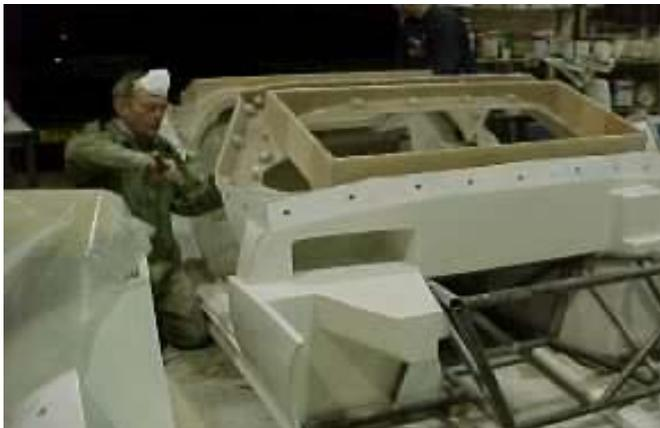
*This picture shows the body buck and mouldings being prepared.*
