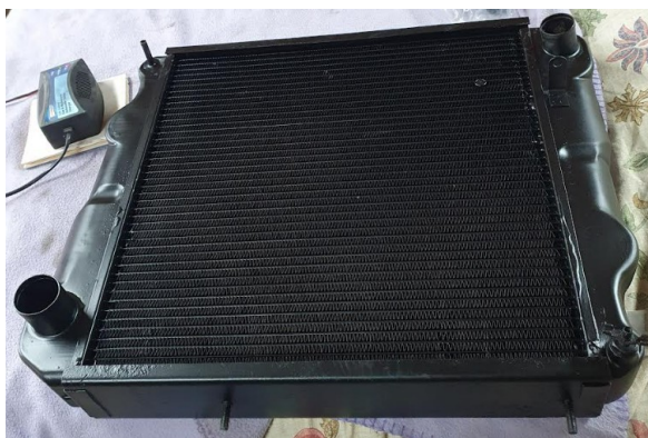
Ed New shiny Radiator re-cored and pressure tested, ready to be fitted
